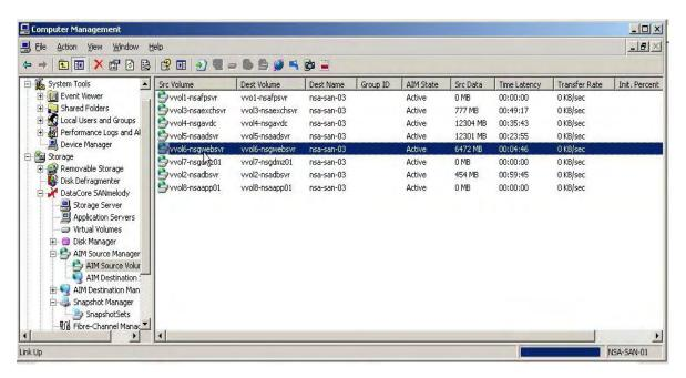
Even with the addition of an extra 6GB to the AIM buffer, the latencies are remaining roughly similar. It is also relevant to consider that the Riverbed appliance takes a short while to "come up to speed" and since this was a mere 6 minutes after initializing the CIFS pass-through command, full speed has not yet been achieved.
