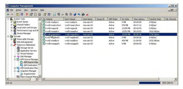
The Riverbed Appliance continued to accelerate the AIM transfer rate, and proof of this is displayed in the following screenshots. The first shows Riverbed passing through the CIFS traffic, and the subsequent DataCore screenshots show the transfer rate improvements as the Riverbed reaches full acceleration, as well as the reduction in source buffer size and a decrease in time latency.
