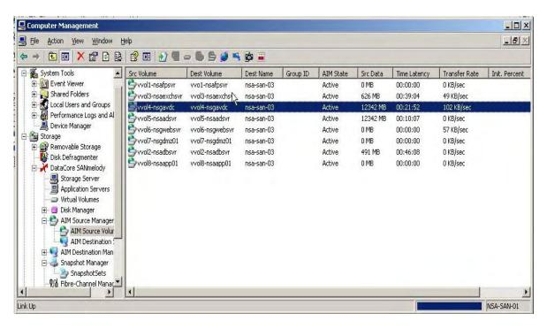
It is also possible to see that the transfer rate has remained relatively constant, implying that since there is more data to be transferred over the link, at a constant rate, the time to catch up will increase. This has potentially serious consequences for the RTO and RPO objectives of the organization, especially in a regulated DR environment.
