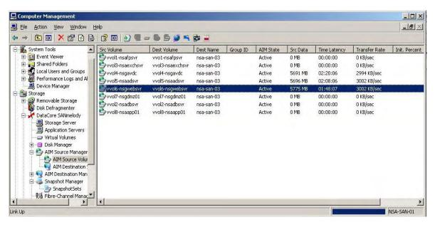
The previous screenshot was taken at 14:33 and the final VM Clone completed its buffering at 12:51. If we subtract the total AIM Src Data figures, to find the volume of data transferred across the link in the 102 minutes we left it processing, we arrive at a figure of 20,063MB or 20.063GB of data transferred in 102 minutes. The full theoretical calculation and the actual transfer calculations are shown below.
