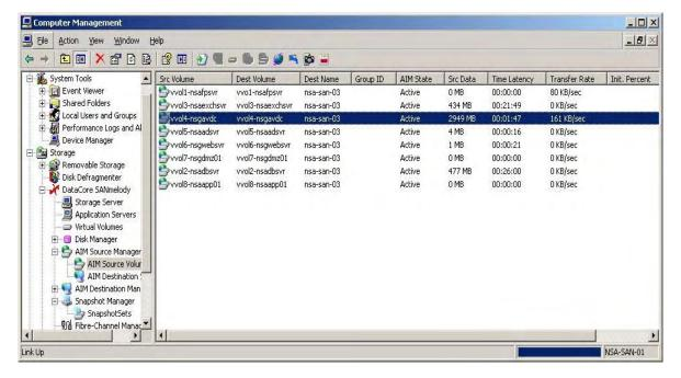
As is evident from the increasing Time Latency below, when competition for the line heats up, it slows down other volumes being remotely replicated. Their latency, which is increasing, measures the disparity between the production and DR site. Were there to be an incident at the production site in this instance, RTO and RPO SLA's could be compromised. This slowing trend continues as the newly created Virtual Machine size continues to grow until it reaches the defined 12GB limit.
