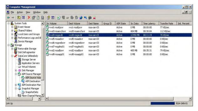
As you can see, by the time the second Virtual Machine has been created and stored, the latency has reached almost 40 minutes, from its initial starting point of 20 minutes and is expected to increase further. Replication traffic for the rest of the production site is also beginning to be affected.
